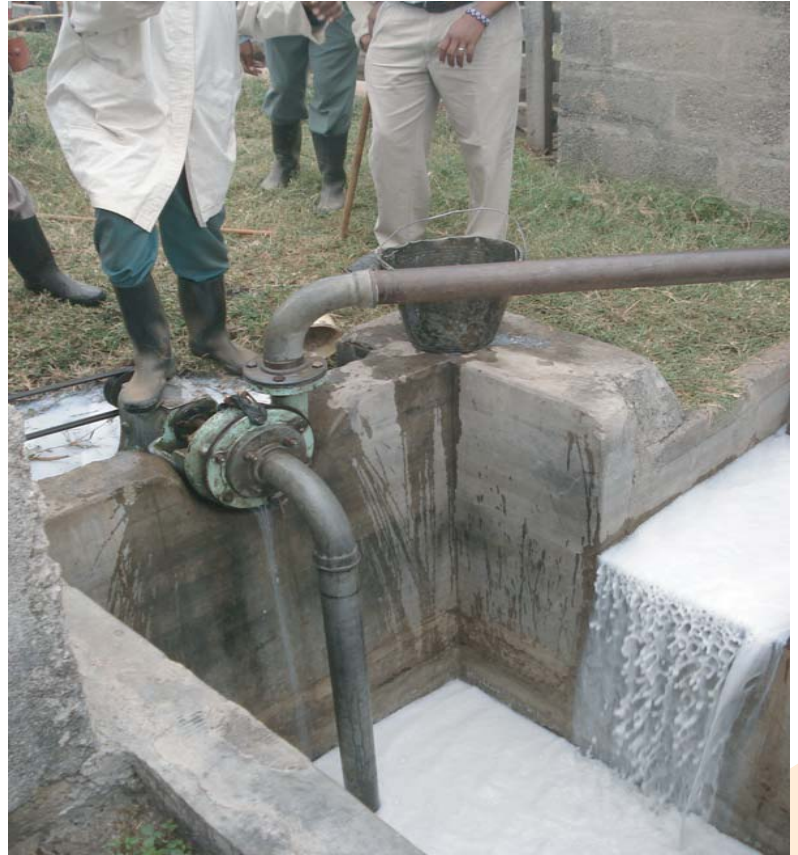
2. A tick spraying pump and sump for the Maasai Rural Training Centre's cattle. This will sell certified crop seeds, farming tools and veterinary supplies to the community.
